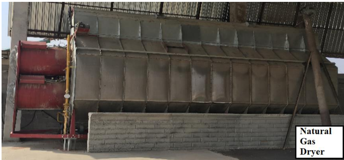
Image 1. Appearance of Natural Gas Industrial Dryer
